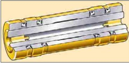
**Cartridge Joints.** Factory-sealed cartridge joints are welded to control end play. They offer improved seal integrity through an innovative new sealing system and do not depend on the link interface to remain sealed. As with all new Cat undercarriage products, they are filled with special oils.
