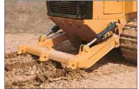
**Ripper-Scarifier.** A radial ripper-scarifier is available for the 953D as an attachment. It is mounted with two pins pressed into each side of the main frame. Two cylinders raise and lower the ripper. The ripper beam has three pockets for holding ripper shanks. The six pins in the linkage do not require lubrication. The 953D ripper-scarifier is intended for ripping frozen ground, asphalt and easily ripped rock. It is not designed for hard rock.
