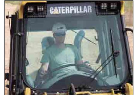
**Viewing Area.** Large windows use tinted glass to reduce glare and provide an excellent view to the bucket, tracks, and around the engine enclosure to the rear.
