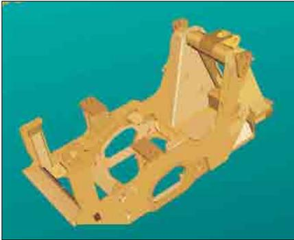
**Mainframe and Loader Tower.** The 953D Main Frame and Loader Tower is a single, slab rails with reinforced crossings, with castings and forgings incorporated at points of high stress, to distribute those stresses over wider areas for long structural life.
