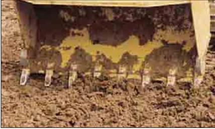
**General Purpose Bucket.** The General Purpose (GP) bucket is designed for excellent loadability and long life in a broad range of applications such as hard bank excavating, stripping and stockpile loading. High-strength, low-alloy steel helps the bucket resist dents and abrasions.
