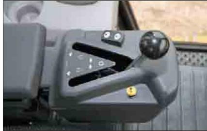
**Travel Speeds.** Travel speeds are infinitely variable between zero and top speed. Two speed modes “work” and “travel”, provide two different speed ranges to best match machine speed and torque to the job conditions for maximum productivity. Maximum travel speed is 10 kph when the switch is set in the travel position.
