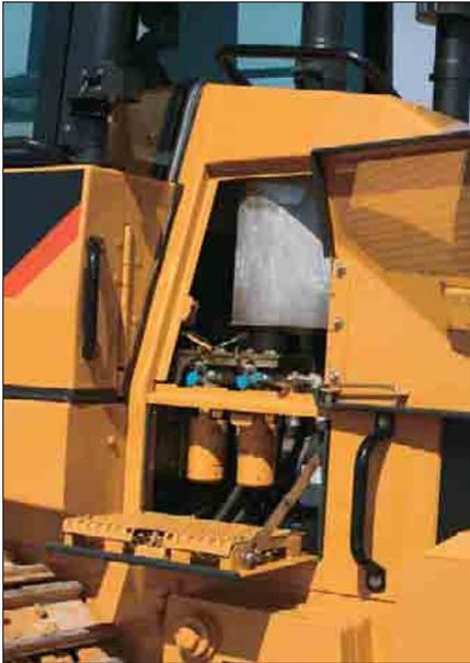
**Left side compartments.** Left engine compartment includes two spin-on hydraulic oil filters that provide filtration for the hydrostatic system. The lower part of the compartment door can be used as a step to access the shunt tank fill, the air pre-cleaner (if equipped) and allows easy cleaning of the rear window.
