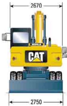
Undercarriage with dozer only
