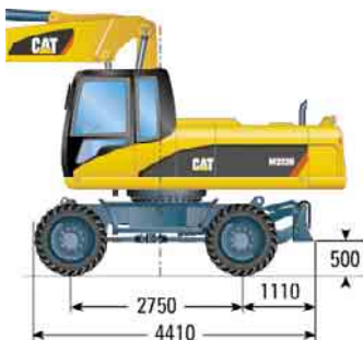
Undercarriage with dozer only
