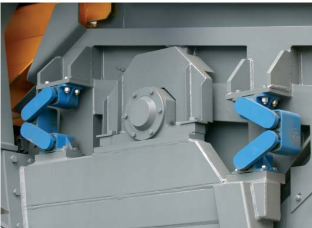
Double deck heavy duty screening unit (Grizzly)
