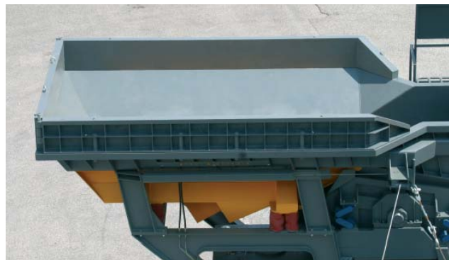
Feedhopper & vibrating chute
