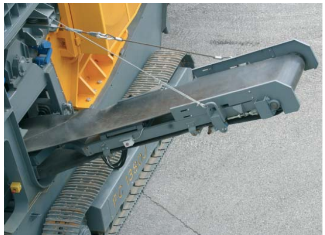
Side conveyor belt
